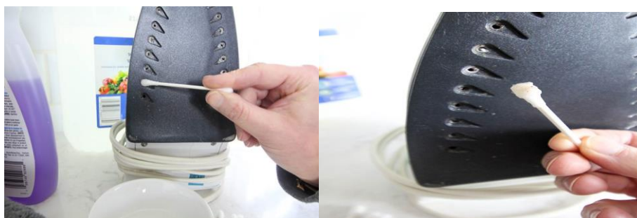
Fig. 2.4: Cleaning of steam vents
