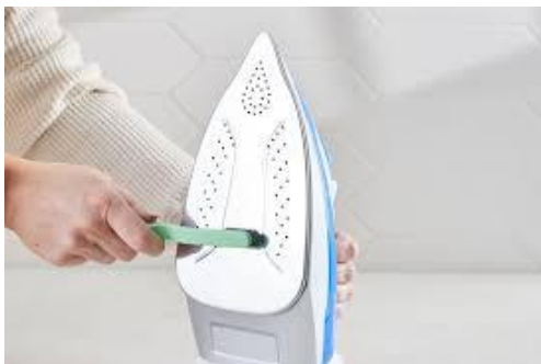
Fig. 2.5: Cleaning of steam vents using toothbrush
