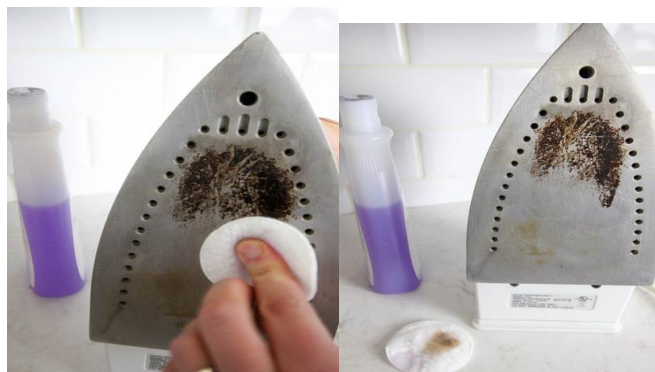
Fig. 2.12: Removal of scorch/burnt marks on electric iron
