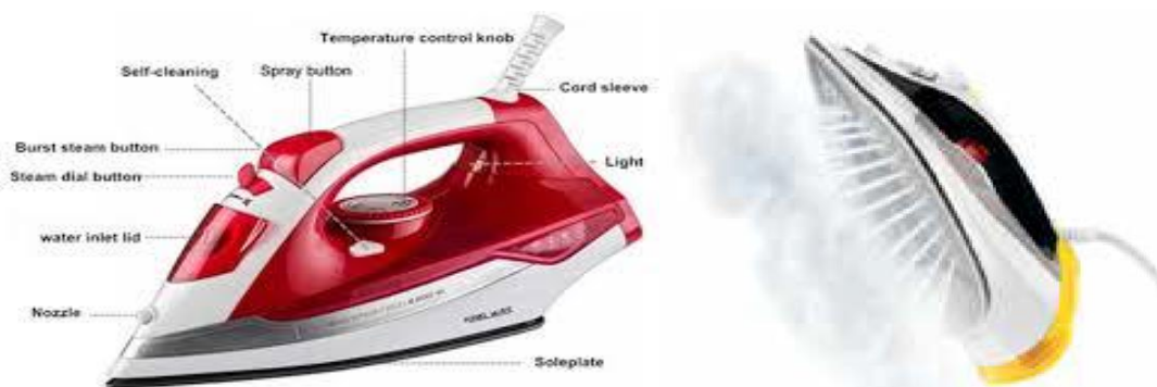
Fig. 1.10: (a) Steam iron parts (b) Steam generation
