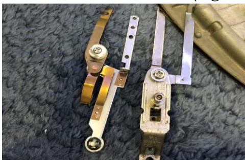
Fig. 2.24: Replace the thermostat
