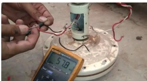
Fig. 1.27: Checking of motor windings
