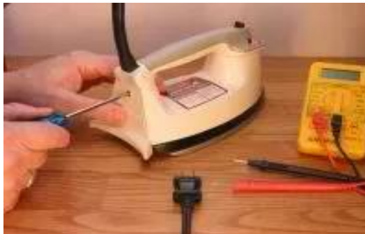
Fig. 1.46: Use multi meter to check iron
