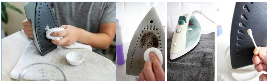
Fig. 1.35: Cleaning the Soleplate
