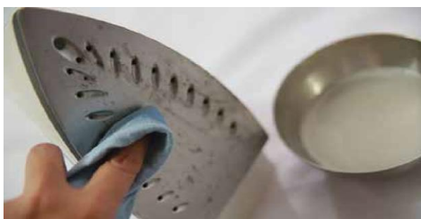
Fig. 2.9: Cleaning of soleplate
