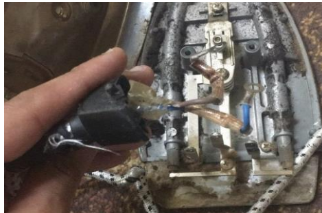
Fig. 2.21: The power cord inside the iron
