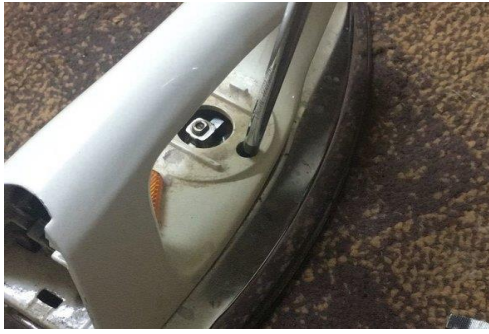
Fig. 2.19: Use the screwdriver to remove the cover panel
