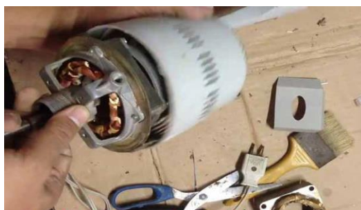
Fig. 2.8: Installing new motor
