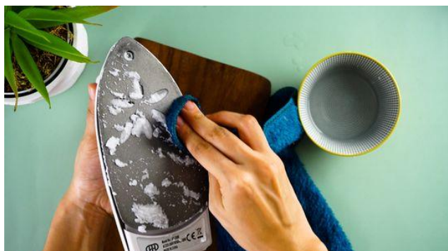
Fig. 2.8: applying the mixture to the soleplate
